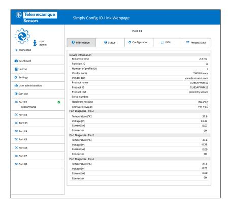
The block **Device information** displays the following device-specific information on this IO-Link device:
