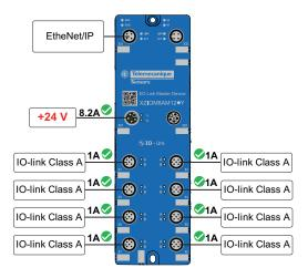
One IO-Link class A device each requiring maximum 1 A current is connected to the ports X1 to X8 of XZIOM8AM12EY. XZIOM8AM12EY requires 0.2 A current.
