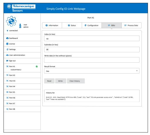
If the access is unsuccessful, the history displays an error message with error codes of IO-Link master and IO-Link device.
