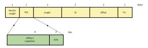
DiffServ is a schematic model for the priority-based classification of IP frames based on an alternative interpretation of the TOS byte. It has been specified in RFC2474.
